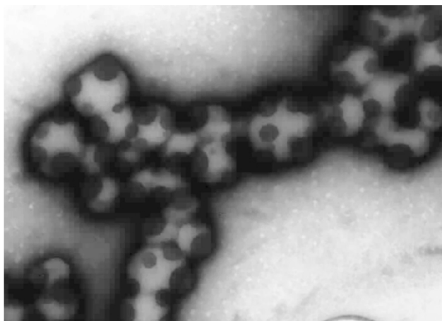
Fig. 6. TEM micrograph of latex CF:VA-ST11 after staining with uranyl acetate and ruthenium tetroxide. This shows the effect of using DDM only in the second-stage styrene polymerization.
